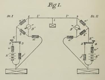
It has also been proposed to use Ruhmkorff's coils for balancing the effect of charge and discharge. This method, however, I believe must be always much inferior to the one of using condensers, inasmuch as the strength of a Voltaic induction current scarcely depends on the speed of signalling, while the charge and discharge of a line, it is well known, is not at all an inconsiderable function of the signalling speed.
