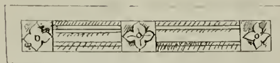
2 feet to 1 inch. Granite block set in over principal doorway
