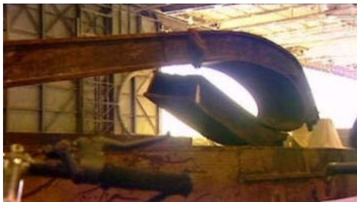
Massive Heat Source Bends Steel Columns With no Buckling
